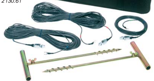
Ground Test Kit for 3-Point testing (supplemental for 4-Point testing) includes carrying bag, two 100 ft color-coded leads, one 16 ft lead and two 16" auxiliary ground electrodes Catalog No. 2130.61
